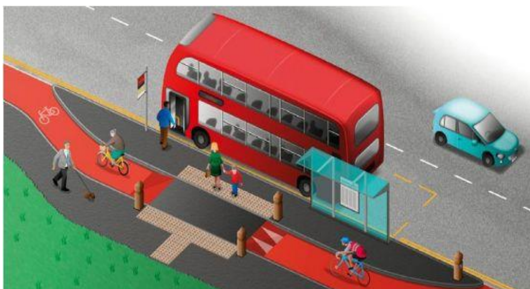
Figure 4.1 Example of a "Floating" Bus Stop
